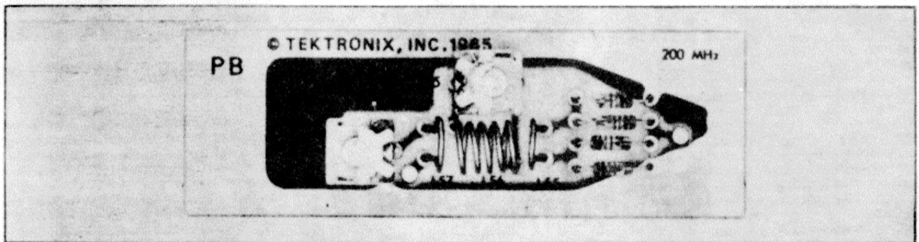
Fig. 4-6. 200MHz (5 ns) etched- wiring board.
